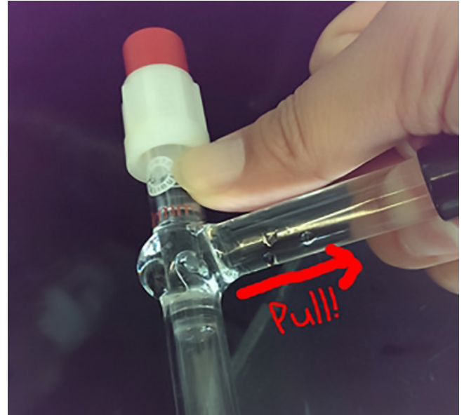
Figure 3: Pulling out air bubbles.
